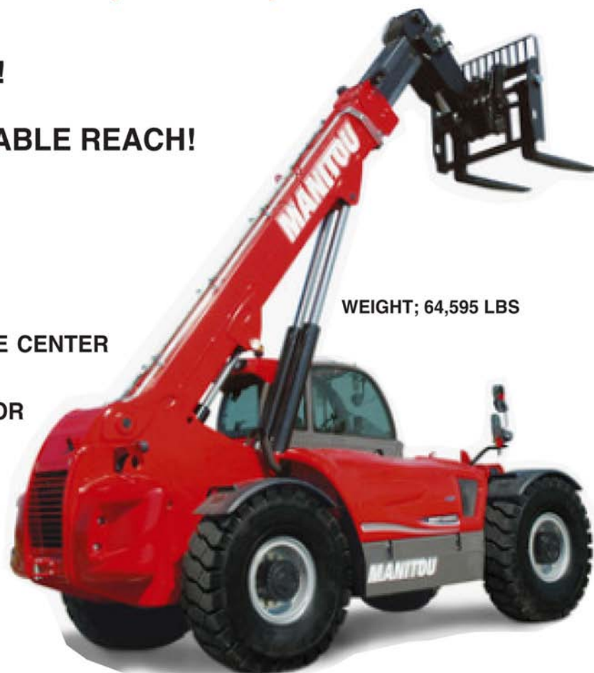
MANITOU MHT 10230 - 50K TELESCOPIC HANDLER LIFTING CAPACITY: 50,000 LBS • LIFTING HEIGHT: 31' 8"
